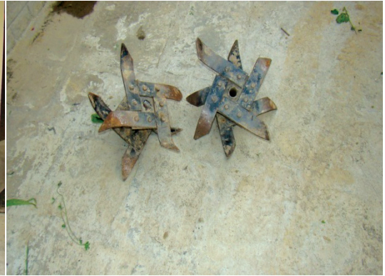
Tiller tines of multi-purpose tiller cum puddler equipment
