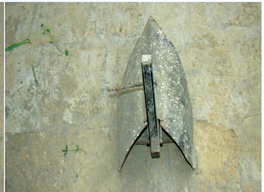
Ridge cum channel maker tool of multi-purpose tiller cum puddler equipment
