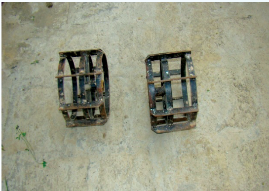
Puddler wheels of multi-purpose tiller cum puddler equipment
